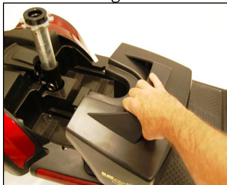
Figure 16. Removing the Battery Pack
