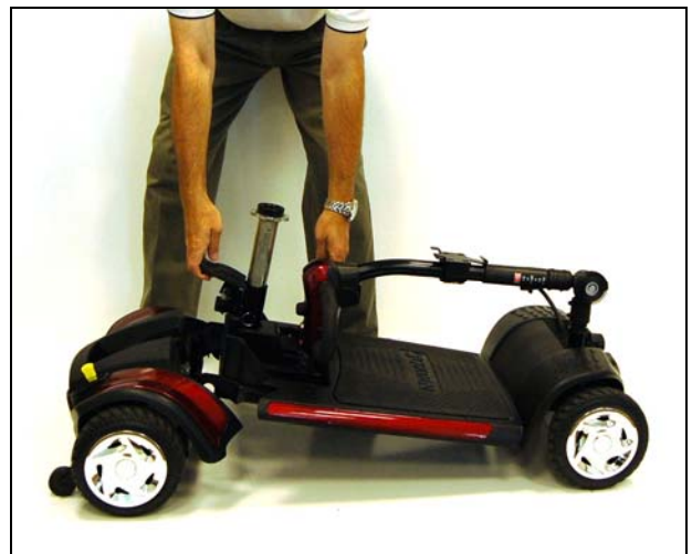
Figure 21. Connecting Frame and Drivetrain
