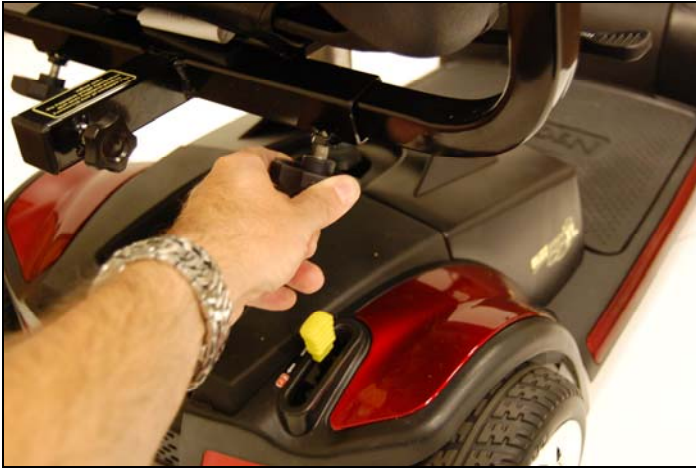
Figure 6. Armrest Width Adjustment
