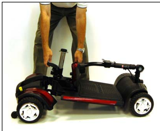
Figure 18. Separating the Drivetrain and Frame
