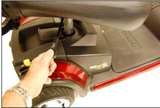
Figure 8: Seat Rotation Adjustment
