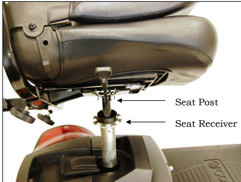
Figure 24. Installing the Seat
