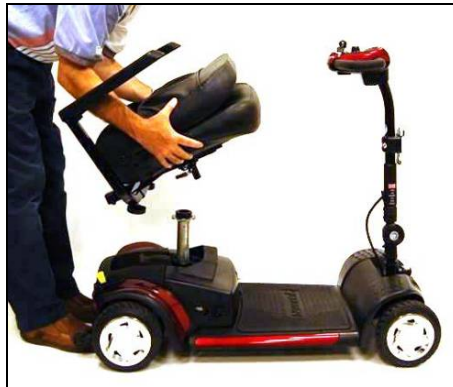
Figure 15. Removing the Seat
