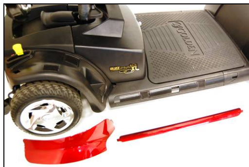
Figure 26. Quick Snap Shrouds Removed
