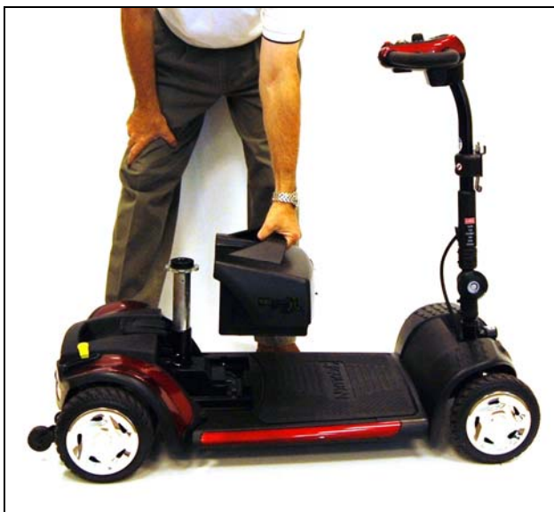
Figure 22. Battery Pack Installation
