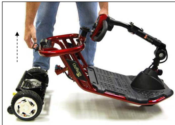
Figure 17. Releasing and Lifting the Frame off the Drivetrain
