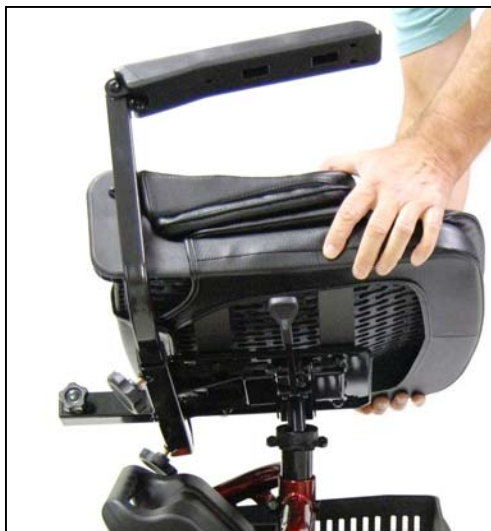
Figure 22. Installing the Seat
