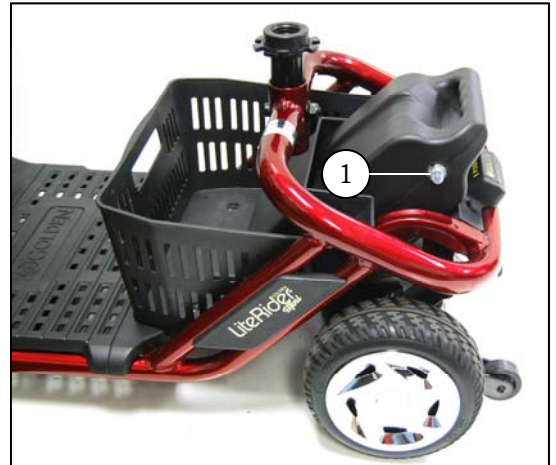
Figure 26. Main Circuit Breaker
