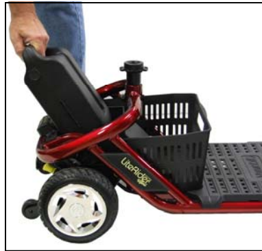
Figure 20. Battery Pack Installation
