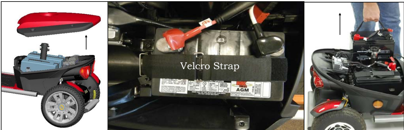
Figure 12. Removing the Batteries
