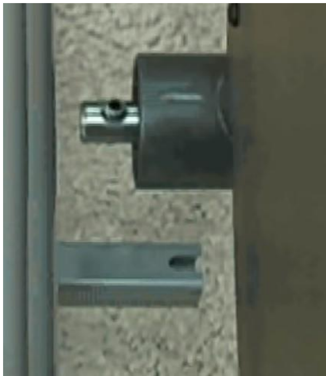
Figure 4. Notched end of drive shaft near cross bar of gear box
